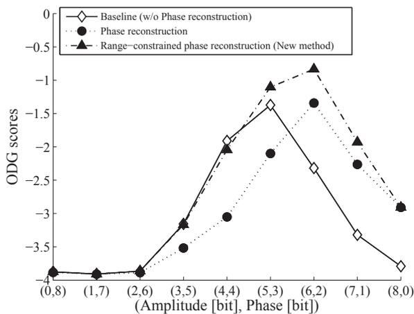
Figure 6: Average ODG scores of PEAQ over ten speech for three different inverse quantization methods
