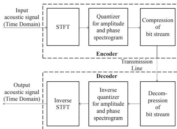
Figure 1: Flowchart of the spectrogram-based audio coding scheme
