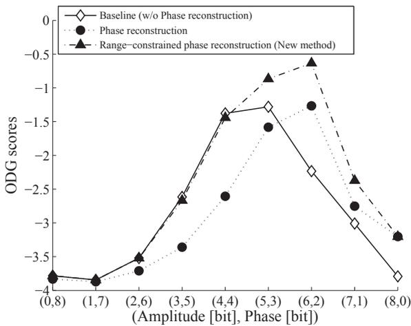
Figure 5: Average ODG scores of PEAQ over ten music excerpts for three different inverse quantization methods
